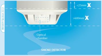
The sensing element of a smoke detection device (optical smoke chamber) should not be less than 25mm below ceiling, and not greater than 600mm below ceiling.
