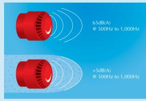
The minimum sound level should be 65dB(A) or 5dB(A) above a background noise which is louder than 60dB(A) (if lasting more than 30 seconds) and at a frequency of between 500Hz and 1000Hz. The maximum sound level should not be greater than 120dB(A) at any normally accessible point. May be reduced to 60dB(A) in stairways, enclosures up to  $60m^2$  and specific points of limited extent.
